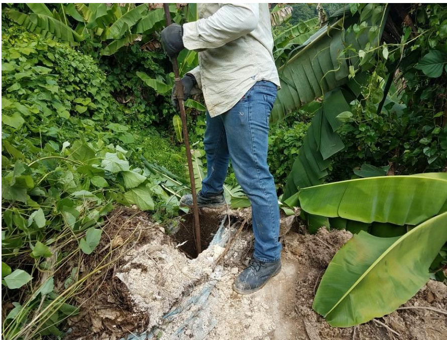
Photograph 6: Hand auger drilling at UIC.
